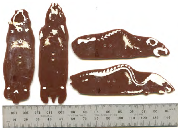
Figure 5. Anatomically correct mouse phantom made by our REU student Leah Turner.
